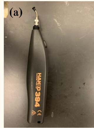
Fig. 1(a) Hakko 394 is used to pick up the microchip from suction
