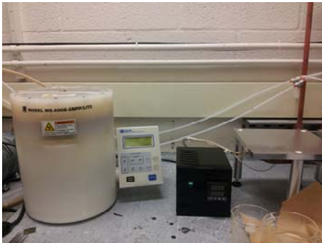
Silicon Wafer is coated with SU-8 and is soft-baked at 95 C
