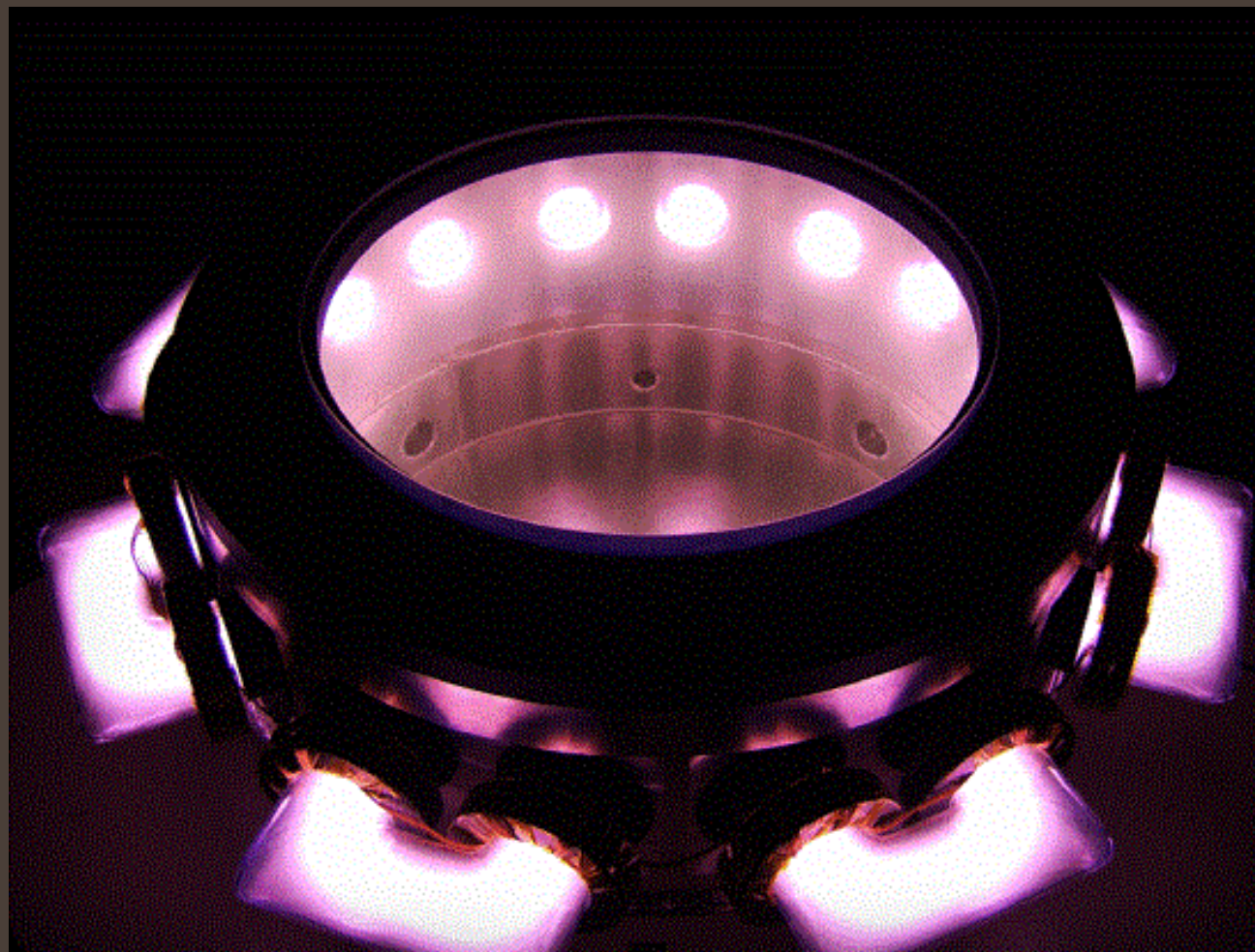
Ferrite ICP design by J. Bang and C. Chung, from Development of Ferrite-Enhanced Side-Type Inductively Coupled Plasma
