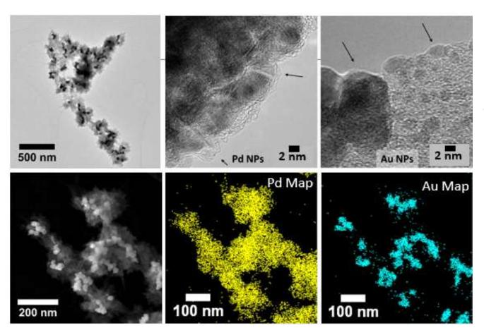
TEM Analysis of Pd/Au Nanoparticles on Graphene
